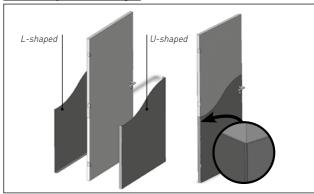
With a thermowelded joint along the door edges
