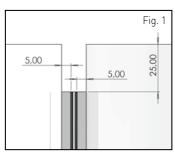
Step 1: position the base plate in relation to the edge of the DECOCHOC panel according to the above dimensions.
