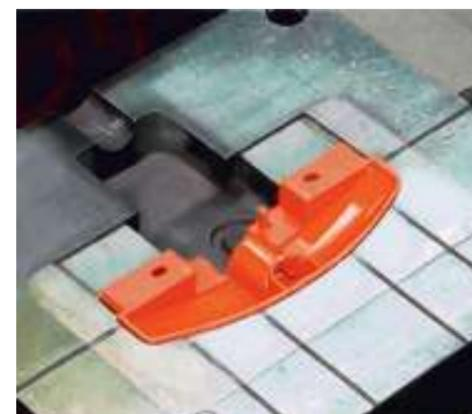
Injection mould - Impact 200 end piece
