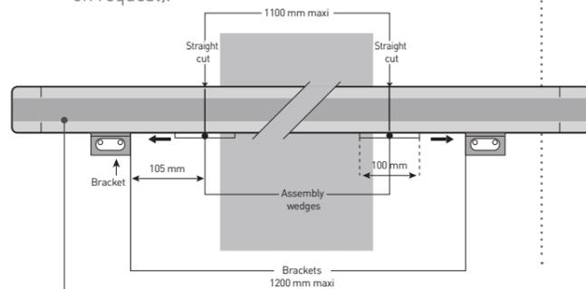
Section of Starline profile (up to 1100 mm), especially machined for service duct. (Other dimensions available on request)
