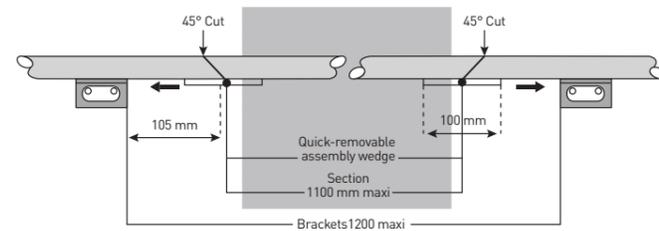
For Escort handrail, Rapid'Access®, the articulated link has been especially designed for service duct, to complete with one quick-removable assembly wedge. (available in chalk or anodised look)
