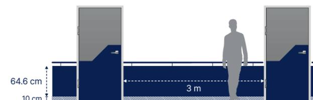
Manage and reuse your offcuts by cutting standard panels at mid-height. 80% of the wall's surface is protected against impacts and tearing.
